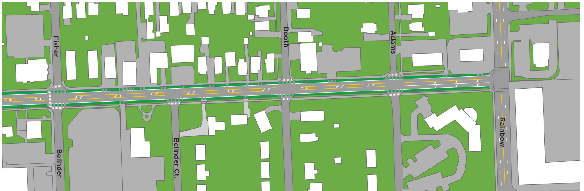
Road diet with protected bike lanes: 47th Avenue from Fisher Street to Rainbow Boulevard.
